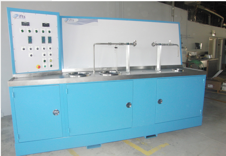
Custom-developed fuel filter test stand in accordance with ISO 4020 standards
